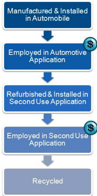
Fig. 1. Lifetime of a PHEV/EV battery when second use applications are considered to increase its total lifetime value.
